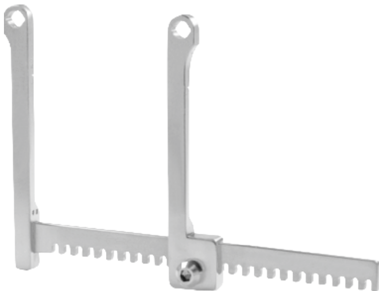
CASPAR UV-342 - 343 Caspar Vertebral Column Retractor for Laminectomy and Hemilaminectomy (Lumbar, Thoracic, Cervical), stainless steel, complete set, 145 mm spread, UV-342 125 mm arms, consisting of UV-343 145 mm spread, hinged includes Screw Driver for spreading bar
